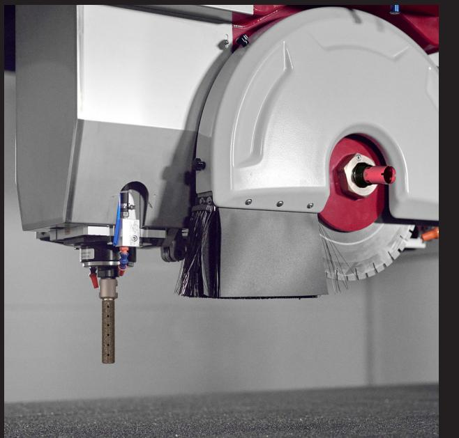
Main spindle with possibility to mount discs up to 600 mm by means of flanges and drilled central axis with hydraulic coupling for drills or cutters. Additional high-speed Rocket Tool spindle (optional) that maximizes the performance of Finger Bit tools.
